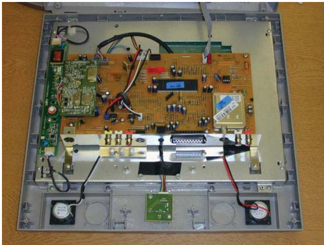
Fig. 3. Mikomi 15LCD25 LVDS link: the thick black cable near top center.
